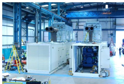
The flexibly coupled IP23 Alternator operating in conjunction with an AVR using 'AREP' + 'PMI' excitation delivers improved transient load performance. Vibration levels are controlled by the heavy duty common base-frame with flexible mounts for the engine and alternator."
